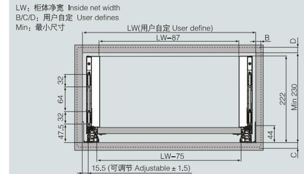
**前接码面板安装尺寸 Connectors front panel dimensions**
