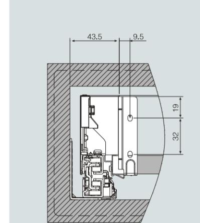
**调节机构 Adjustment mechanism**
