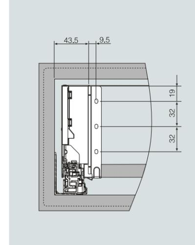
**调节机构 Adjustment mechanism**
