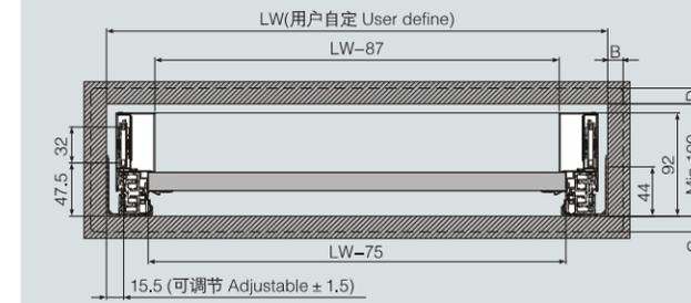
**前接码面板安装尺寸 Connectors front panel dimensions**
