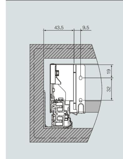
**调节机构 Adjustment mechanism**
