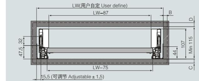
**前接码面板安装尺寸 Connectors front panel dimensions**
