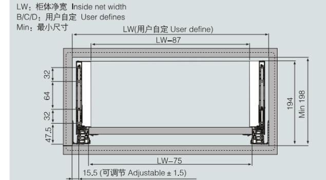
**铝面板装配示意 Aluminum front panel assembly**
