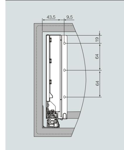
**调节机构 Adjustment mechanism**
