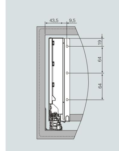
**调节机构 Adjustment mechanism**
