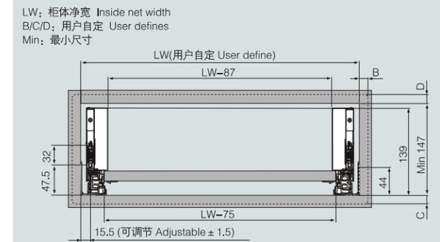
**前接码面板安装尺寸 Connectors front panel dimensions**
