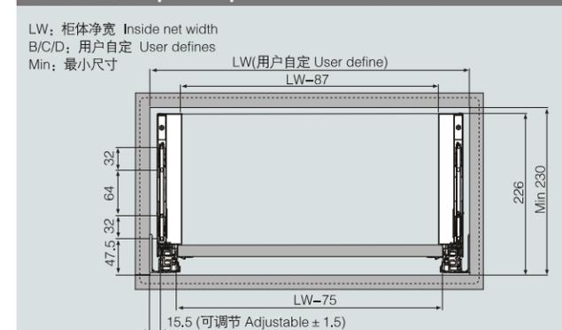
**铝面板装配示意 Aluminum front panel assembly**
