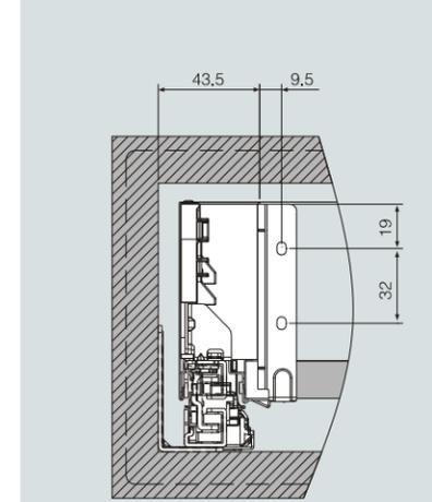
**调节机构 Adjustment mechanism**
